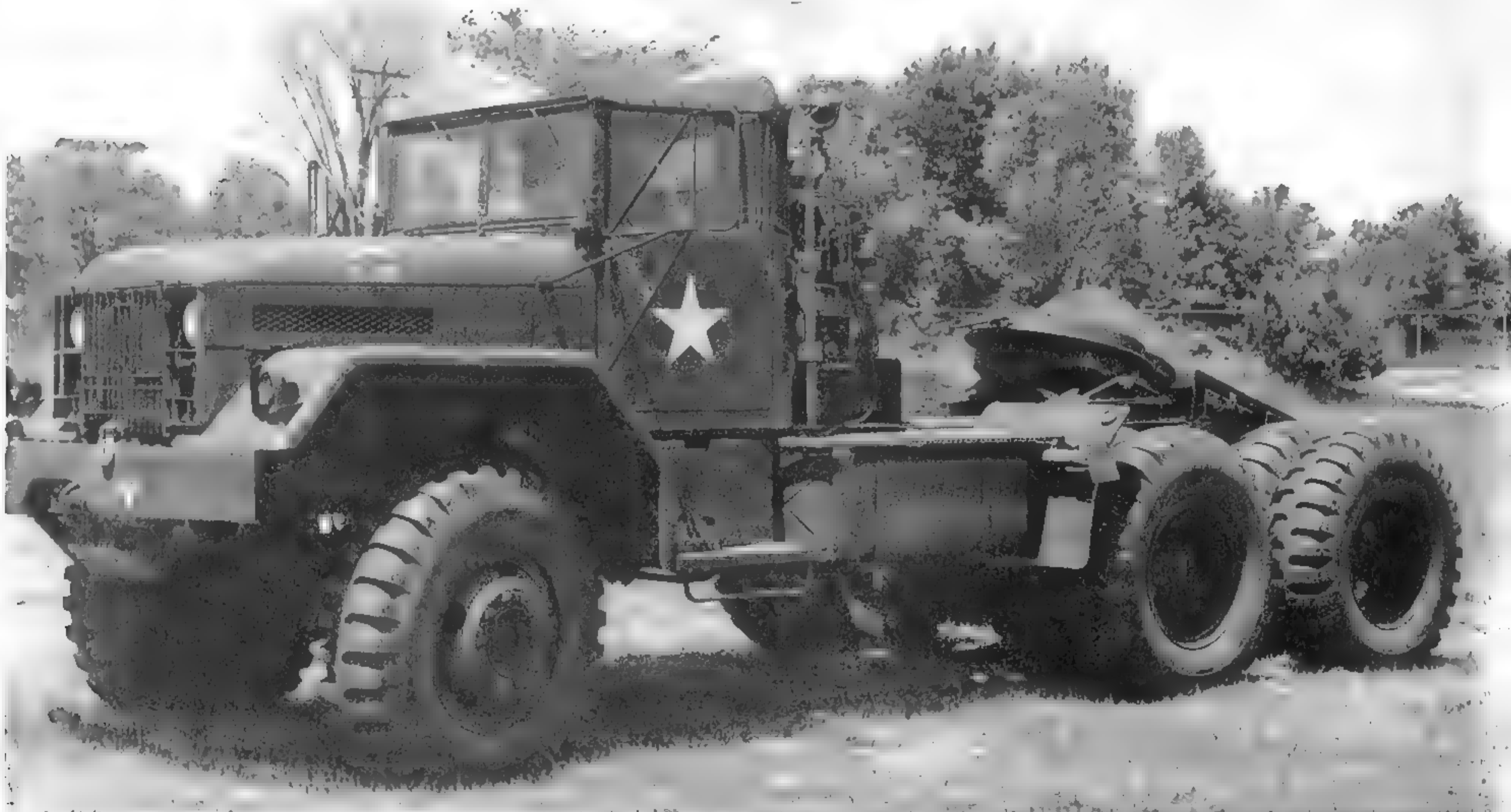
This tractor has a single rear winch and the high-mounted fifth wheel. The trailer these tractors were originally intended to pull, the M15A2, was designed for use with the WWII-era M26 Pacific, which used the same 14-24-in. tires as the M123. While the top frame rails of the M123 are approximately level with the tops of the tires, on the Pacific the frame is taller than the tires. Thus, the M123's fifth wheel was raised to provide a level ride attitude of the trailer. Later M123 models were used with different trailers and the raised fifth wheel was no longer needed. (U.S. Army photo)
